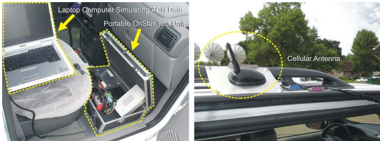
Figure E-3. Portable OnStar Test Unit in Support of Voice Routing Field Test
