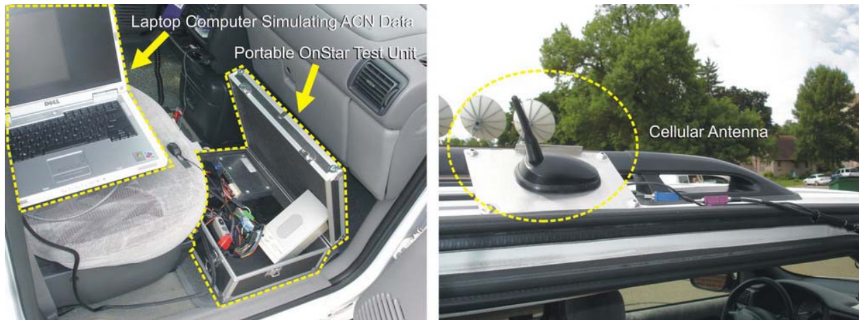
Figure 3-1. Portable OnStar Test Unit in Support of Field Test
